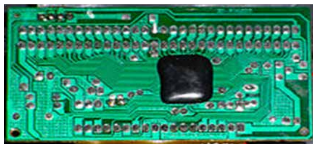
Figure 2: Printed circuit board with glob-top protected IC
