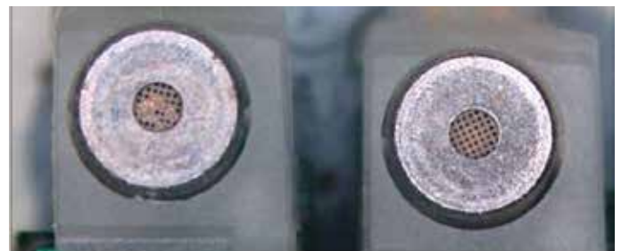
Figure 6 shows the difference in debris build-up on the microphone inlet screen for non-nanocoated (left) vs. nanocoated (right) devices that went through the AST test.
