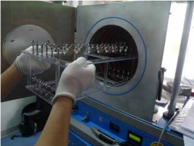
Figure 5: Hearing instruments mounted in fixture being loaded into the processing chamber.
