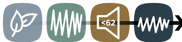
Figure 2. The Soft Level Noise Reduction system will suppress noises below 62 dB SPL, without affecting other soft sounds like soft speech.
