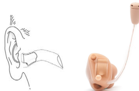
Figure 1: The placement of the microphone in the concha cymba hides the microphone not only for improved cosmetics but also for improved acoustic performance due to pinna effects.
